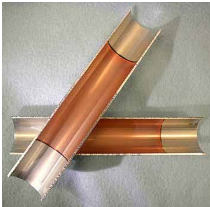
Figure 2. Inside of a copper-coated target cylinder.
