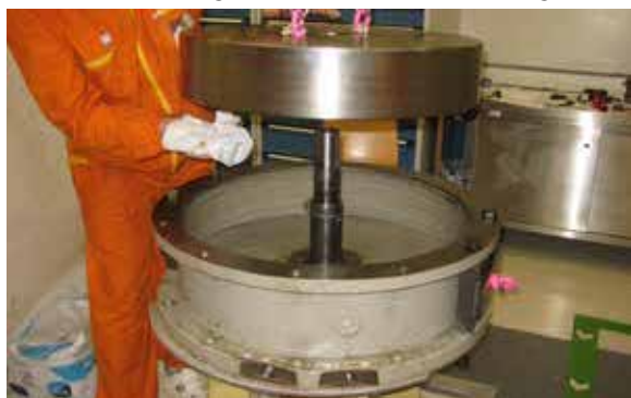
Figure 2: Removal of the flywheel for the exchange of a bearing at a primary pump.
