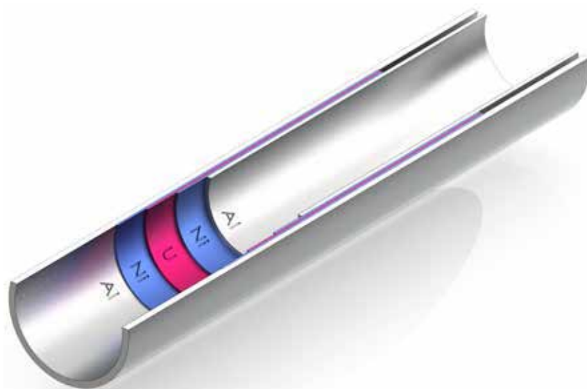
Figure 1. Sectional drawing of a cylindrical Mo-99 target.
