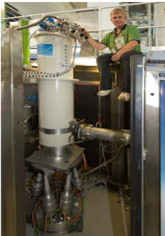
Figure 16: The compensated, vertical 5 Tesla cryomagnet with the new hexapod at KWS-1.
