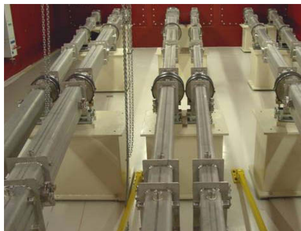
Figure 3: Neutron guides inside the neutron guide tunnel.
