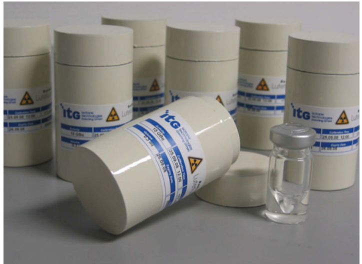
Figure 3: ^{177}\text{Lu} produced by the company ITG at the FRM II at the capsule irradiation facility. The radioisotope is filled in little vials with a volume of 2 ml and then packed in cans with a diameter of 45 mm and a height of 70 mm.
