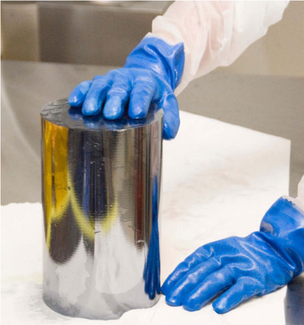
Figure 1: A silicon crystal after the doping at the FRM II neutron source.
