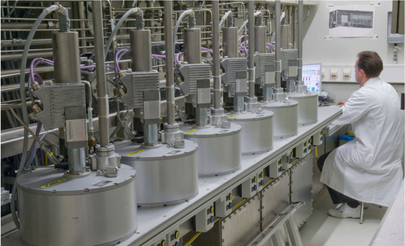
The standard rabbit irradiation system has six independent irradiation channels and is operated by carbon-dioxide.
