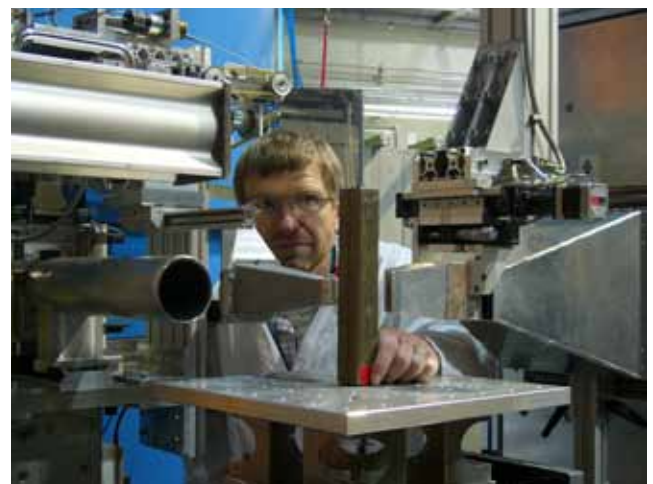
Figure 2: Michael Hofmann using the residual stress and texture diffractometer STRESS-SPEC to study batteries.
