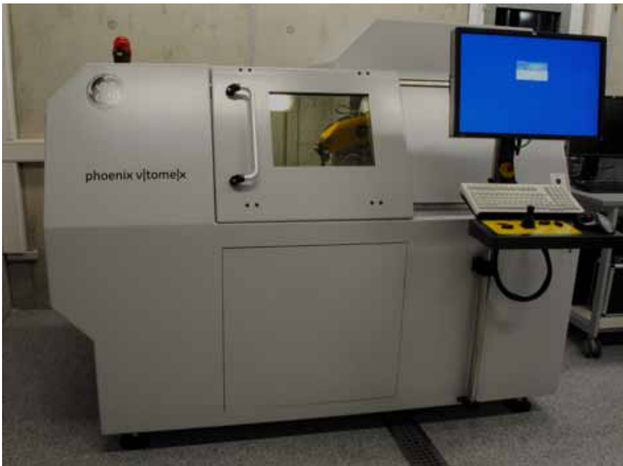
Figure 1: The new high resolution computer tomography facility.
