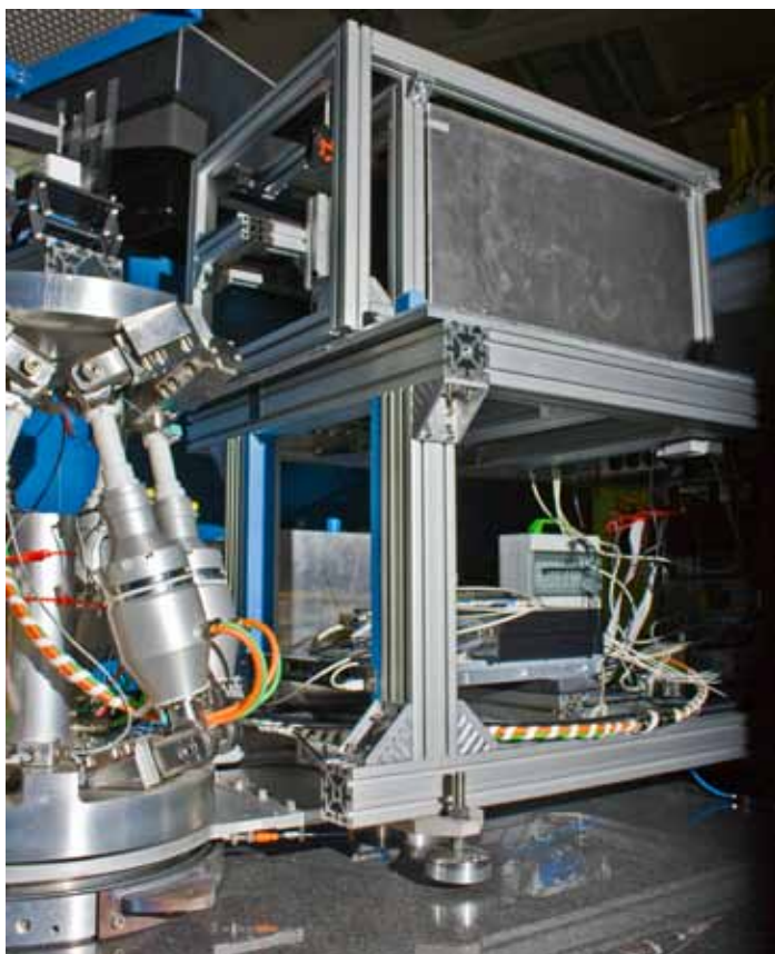
Figure 1: The sample position of MARIA with hexapod, ^3\text{He} -SEOP-analyzer and detector.
