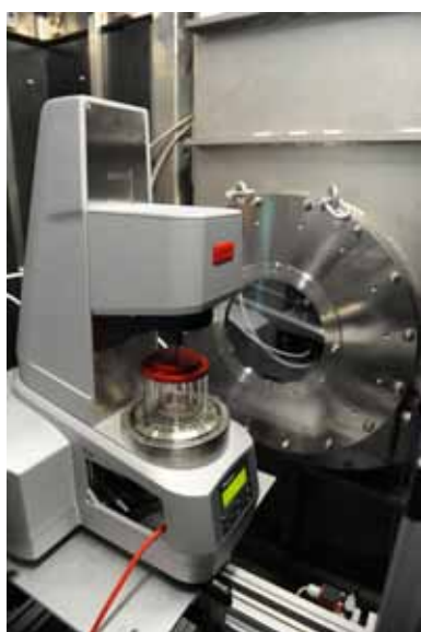
Figure 3: (a) The new Searle rheometer installed at KWS-1. (b) Scattering pattern of an aligned hexagonal cylinder phase of a microemulsion. Second order peaks indicate the high degree of order.
