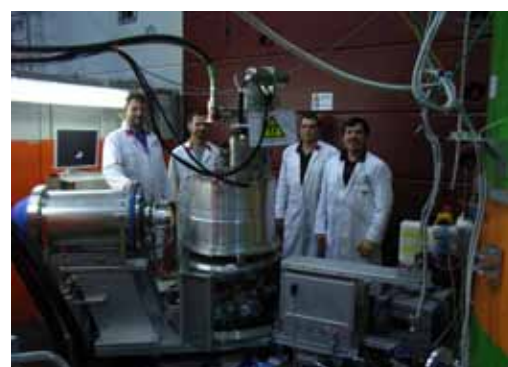
Figure 5: Technical feasibility study, test of the FRM II 7.5 T magnet on-site with POLI.
