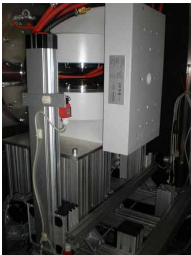
A new Searle rheometer was taken into user operation. The first experiments aimed at microemulsions in a liquid crystalline state where cylindrical micelles on a hexagonal lattice are formed. At a shear rate of 100\text{s}^{-1} we managed to align the sample macro-
